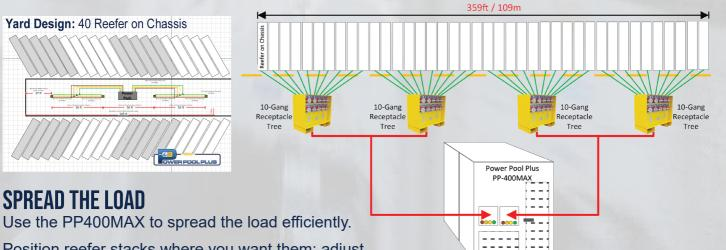
Use the PP400MAX to spread the load efficiently.
